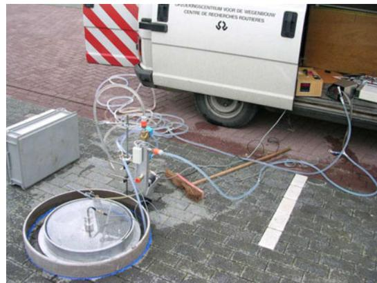
**Figure 6. Double ring infiltrometer**
