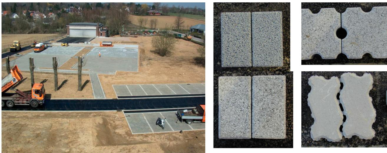
**Figure 3. Overview of the test parking area – porous pavement blocks, pavement blocks with drainage holes, pavement blocks with enlarged joints, classic pavement blocks**
